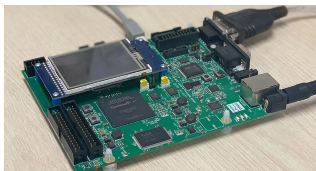
Fig. 2. ARM V2M-MPS2+ FPGA prototyping board
