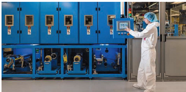
FIG 2 Solid Power’s fully automated, roll-to-roll SSB production facility. (Source: Solid Power; used with permission.)
